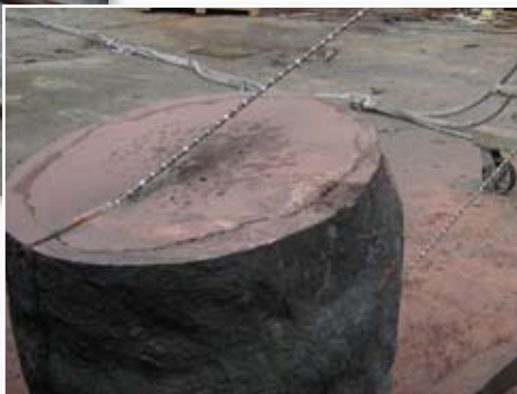
Notice the smooth finish made by diamond wire saw in the photo above.
