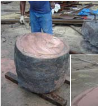
Notice the smooth finish made by diamond wire saw in the photo above.
