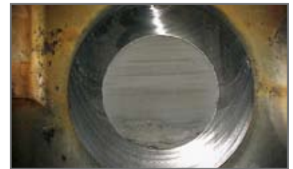
Fig. 9. Note smoothness of wire cut.
